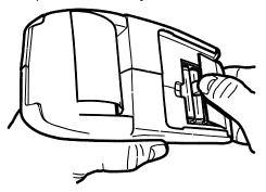
3. Insert four (4) AA Rechargeable (preferred) NiCad, NiMH, or Alkaline batteries to positive and negative connectors as indicated.
